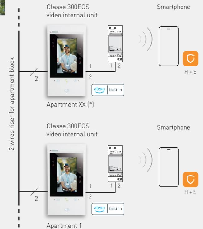
**NOTE:** For the sizing of multi-family systems refer to the General Installation Standards of the 2 Wire System Technical Guide.
